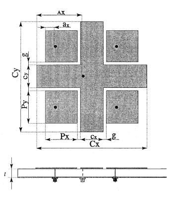
Figure 5. The geometry of the cross-subarray patch antenna.
