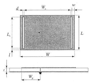
Figure 2. The geometry of the slotted rectangular-patch antenna.
