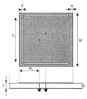
Figure 3. The geometry of the slotted square-patch antenna.
