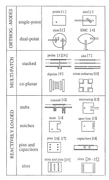
Figure 1. Dual-frequency patch antennas.
