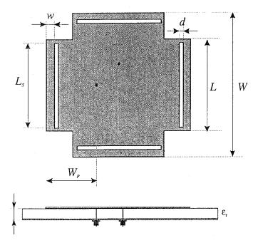
Figure 4. The geometry of the slotted cross-patch antenna.
