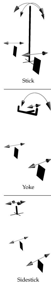
Figure 1.12: Some standard pilot controls: the rudder pedals are almost universal for yaw control, but the pitch and roll controls can vary markedly between aircraft
