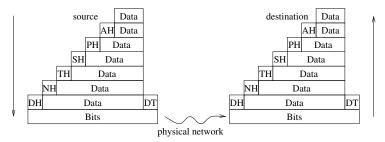
Data is encoded and decoded
