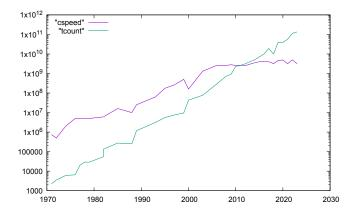
Log of speed and transistor count against date of Intel processors
