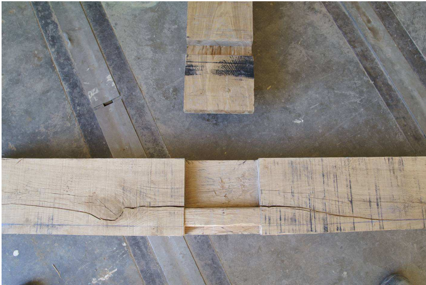
Cog joint after test
