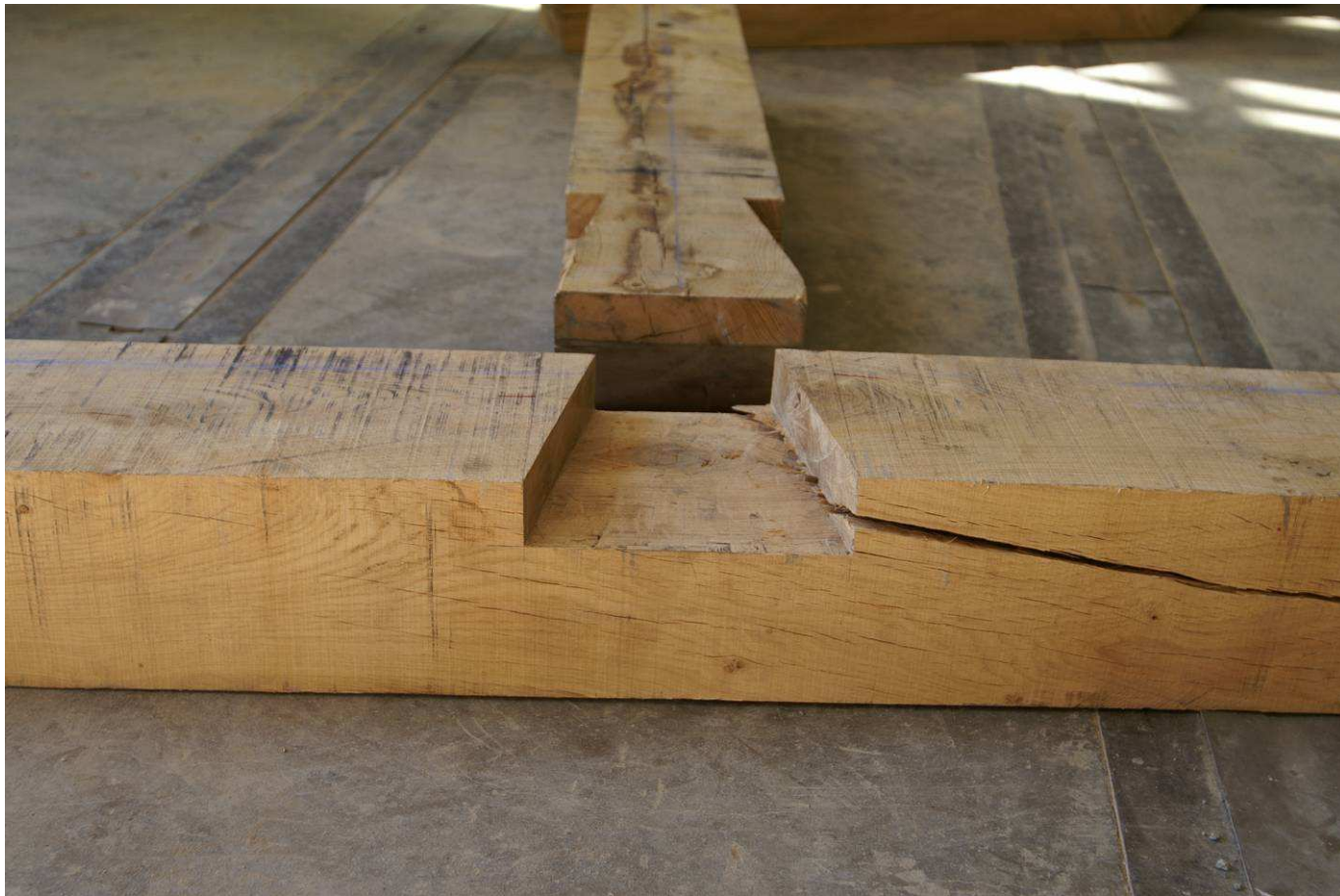
Lap dove tail after test
